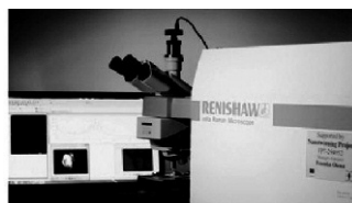
InVia micro-Raman spectrometer with lasers \lambda = 786 and 633 nm (Renishaw, England)
